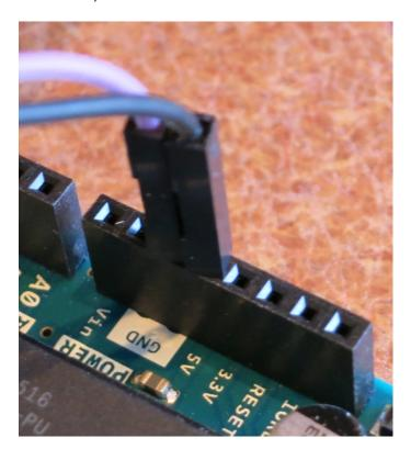
**5-a.** Mount the buzzer either directly to the Arduino as shown here,
