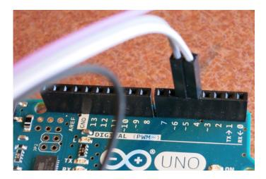
**4.** Connect ground to ground. (The wire shown here on the left.)
